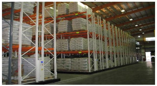
The mobile pallet racking solution, is the optimal solution for storage. Helping to reduce costs for a new building or the possibility to better utilize existing storage space more efficiently.
